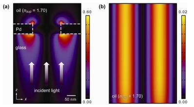
Fig. 2. Simulated electromagnetic field distributions  $(|E_z|^2)$  at a RA-SPP minimum ( $\lambda = 628$  nm). (a) SPPs are visible on both sides of the Pd hole array film, where  $n_{sub}$  (glass) = 1.52, and  $n_{sup}$  (oil) = 1.70. (b) RA at z = 200 nm above the film, where SPPs have significantly decayed.
