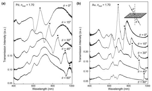
Fig. 4. Angle-resolved transmission spectra of (a) Pd and (b) Au subwavelength hole arrays with  $n_{sup} = 1.70$ . The RA-SPP resonance ( $\bigstar$ ) in Pd shifted with  $\theta$  but did not change much in amplitude and peak width, whereas the intensity of the RA-SPP peak in Au hole arrays dramatically decreased with increasing  $\theta$ .
