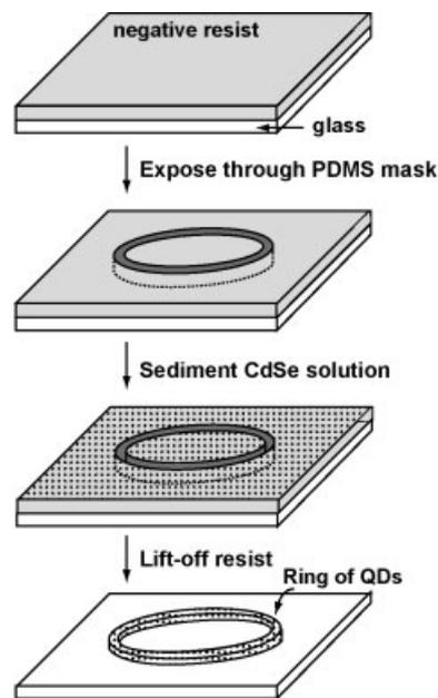
**Figure 1.** Schematic illustration for patterning chemically synthesized nanomaterials using templates made of photoresist. A pattern is produced in negative-tone resist using PSP with composite PDMS masks. The scheme depicts an example of a ring generated by PSP using a mask patterned with circular, recessed posts. The nanomaterials assembled into the recessed regions of the template by sedimentation. Removal of the photoresist generated arrays of structures in specific patterns.
