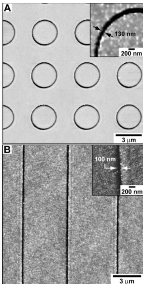
**Figure 2.** AFM images of A) rings and B) trenches formed in negative tone resist using phase-shifting photolithography. These line widths can be as narrow as 100 nm.
