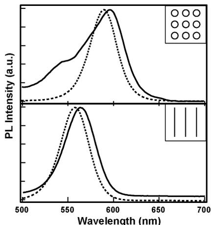
**Figure 4.** Photoluminescence (PL) spectra of CdSe/ZnS nanocrystals in aqueous solutions (dashed lines) and patterned on substrates (solid lines) from Figure 3. Both A) larger dots patterned into rings and B) smaller dots patterned into lines exhibited a red-shift in the PL compared to the same dots in dilute solutions. The insets represent the mesoscale patterns of the CdSe/ZnS dots from which the PL was measured.
