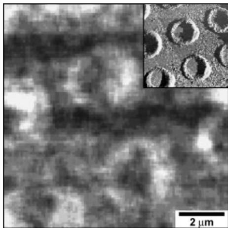
**Figure 5.** Fluorescence NSOM image of arrays of quantum dots patterned into ring structures. Inset: Amplitude image of rings of CdSe/ZnS dots acquired in constant-force mode.
