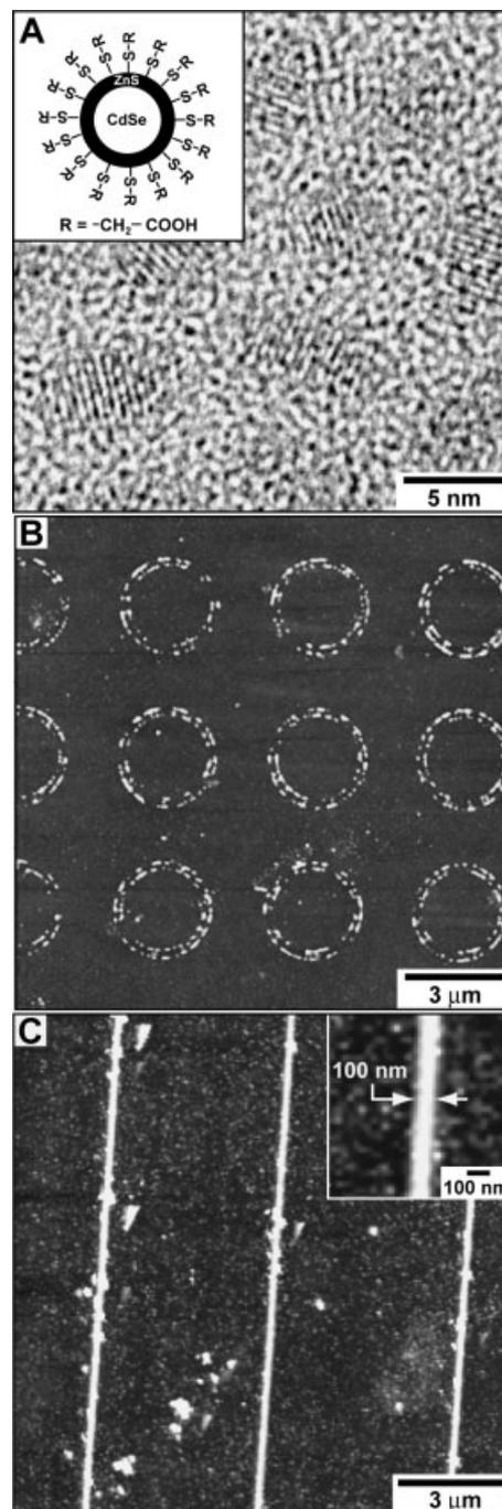
**Figure 3.** A) TEM image of crystalline and slightly oblong CdSe nanocrystals. Inset: Scheme for water-soluble CdSe/ZnS dots. B,C) AFM images of quantum dots patterned into rings and lines using the templates from Figure 2. Lines with well-packed quantum dots were as narrow as 100 nm, and the height of the quantum dot structures varied between 15–50 nm.
